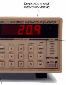
**Each** channel may be independently configured for thermocouple type, display units, and nominal temperature. The first four channels can drive rear panel analog outputs with variable offset and gain.
