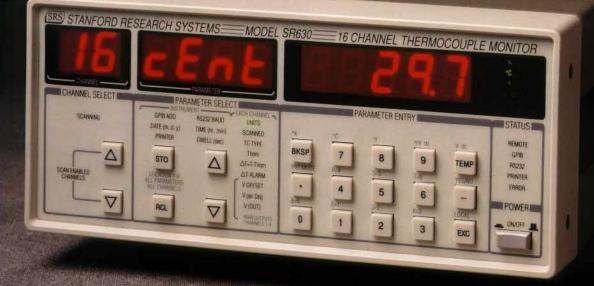
The configuration paramet being changed is clearly displayed to eliminate input errors.
